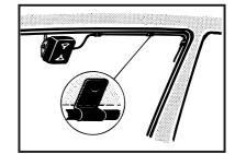
6. Fit matching unit by pressing it firmly into position. Secure cable using clips provided.
