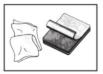
Clean both sides of the windscreen, where the antenna mount and the matching unit are to be fitted, and then remove the protective foil from the antenna mount.
