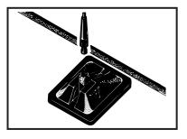
4. Fit the cover and press down firmly. The antenna whip can now be fitted.
